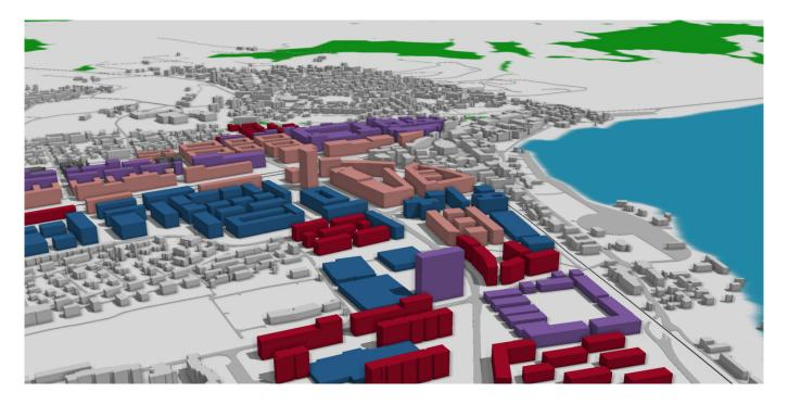
Swisstopo instructed EBP to calculate the building heights of Switzerland from DOM, DTM-AV and VECTOR25 building footprints. The EBP calculation methods enabled the building heights to be calculated quickly from the billions of laserscanning points of the height model. Swisstopo is marketing the building heights record as a new product under the name SwissBUILDINGS3D.
